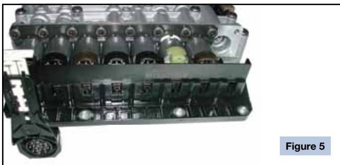
With solenoids cleaned, tested or replaced, this completed assembly awaits installation and will require a re-learn procedure.
