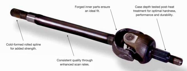
And not only are our axle shafts fatigue-tested to ensure consistent quality, 100% of our front axle parts are ultrasonically tested, so we're able to check for any internal cracks that regular magnetic testing can't reach. We're proud of our quality and consistency testing methods that also meet or exceed market standards—because when it comes to the performance of Spicer axles, there's no room for compromise.
