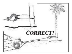
Avoid continuous pulls from extreme angles as this will cause the wire cable to pile up on one end of the drum (*Figure 3*). This can jam the wire cable in the winch causing damage to the cable or the winch.
