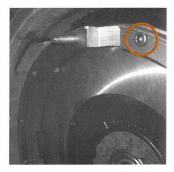
3 Insert two socket screws into the intermediate ring and torque 20-30lbs.
