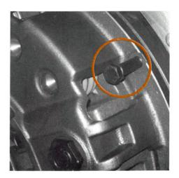
10 Insert clutch mounting bolts into cover assembly, remove the two alignment pins and replace with mounting bolts. Torque to 50 to 55lbs in a criss-cross manner.
