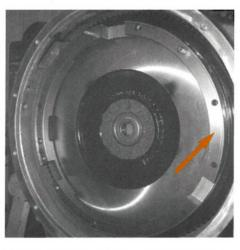
Install intermediate ring onto guide studs making sure it's the correct way.
