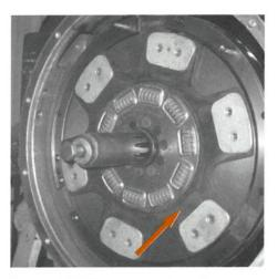
8 Install (PP) pressure plate disc against intermediate plate face through alignment shaft.
