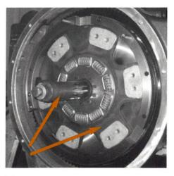
5 Insert alignment shaft and install flywheel disc (FW) against flywheel through the alignment shaft.
