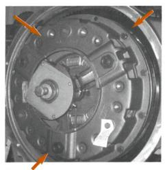
9 Next lift cover assembly and install onto alignment shaft, making sure the three recesses in cover assembly align with intermediate plate lugs.
