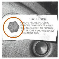
11 Remove shipping bolts, making sure alignment tool is still in place.
