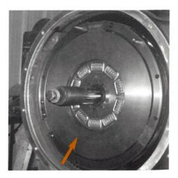
6 Install the intermediate plate in the intermediate ring making sure intermediate plate markings are followed. Make sure the intermediate plate moves freely and the clearance between the intermediate ring drive slots are checked. A clearance of .003" to .007" is required on each side of drive lug.
