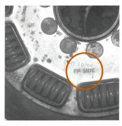
7 Check pressure plate disc (PP) for correct markings.
