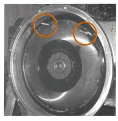
Make sure flywheel and spigot bearing are in good condition. Install two guide studs into clutch flywheel mounting bolt holes.
